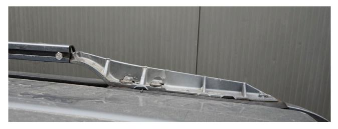
**If your vehicle has no fixed points:** Assemble roof rails with brackets, and place them on both sides of the roof of your vehicle to mark drill holes. Use the rails and brackets as a template. Make sure both sides are similar. Measure twice, double-check, and drill once.
