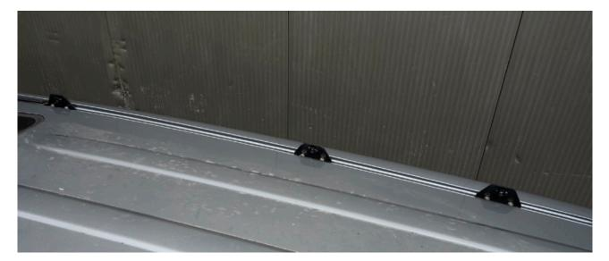
Install appropriate roof rails using M8 bolts included for each of the brackets. Hand tighten only.
