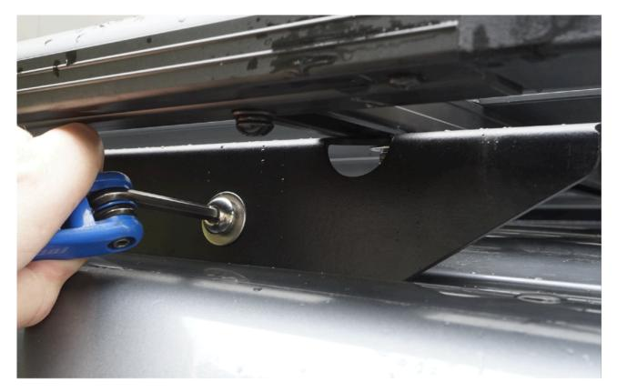
Center the platform on the vehicle roof and tighten all the mounting bolts. Recheck all the fasteners after approximately 100 km.
