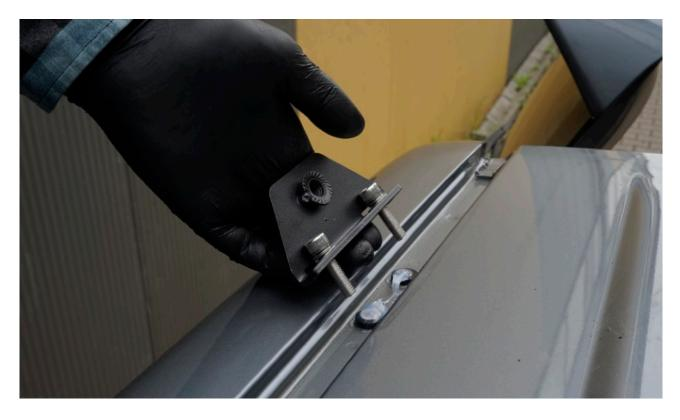
Tighten both bolts all the way in. Make sure to fasten both bolts fairly simultaneously to avoid any miss alignment.
