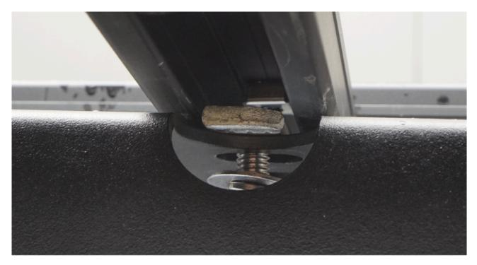
Rotate the T-Nuts 90 degrees to make sure they will lock. Tighten the bolt flush with the locking washers. Don't tighten fully just yet.
