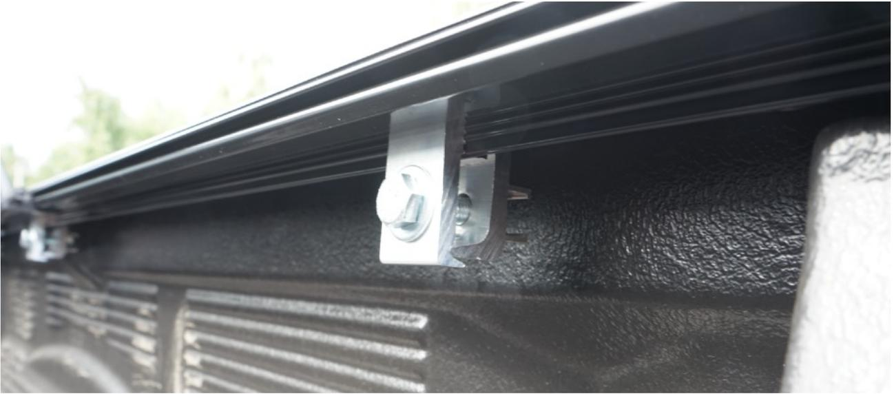
Tighten evenly each clamp while making sure the rail stays level. Check for any unwanted movement. **Continue on page 5.**
