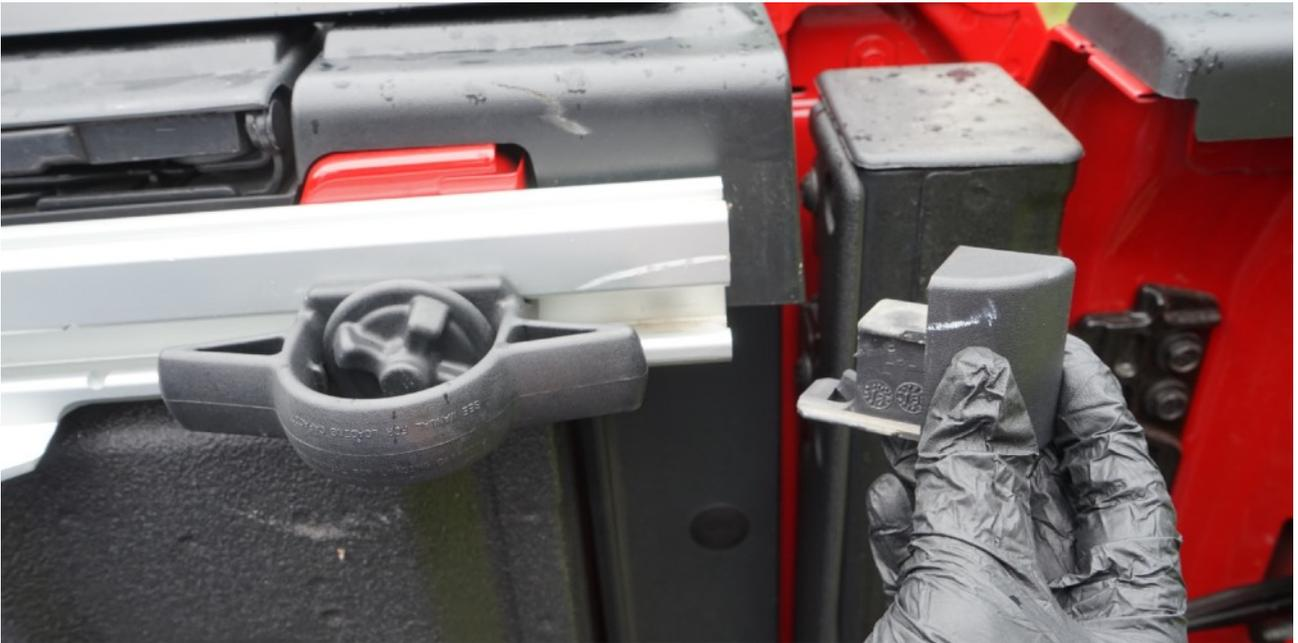
Insert provided blocks and slide them into the rails. Reinstall the end cap.
