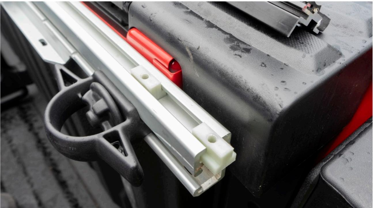
Position the bed cover rail alongside the bed edge and align the blocks to match the openings.
