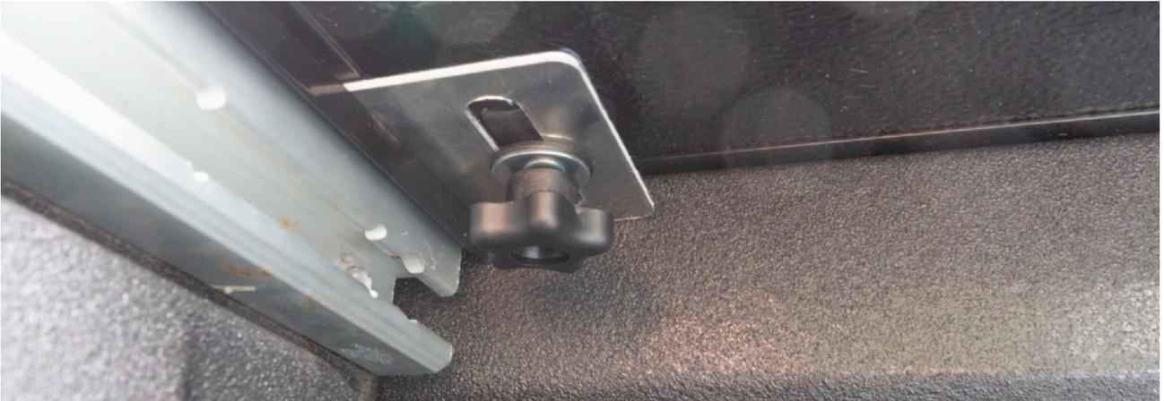
Unfold at least two parts of the bed cover and check for proper side-to-side alignment. Once happy with the position close the tailgate and unfold the whole cover. Check for proper alignment front to back. Check again on all sides, and fully tighten the bolts mentioned in the step before.
