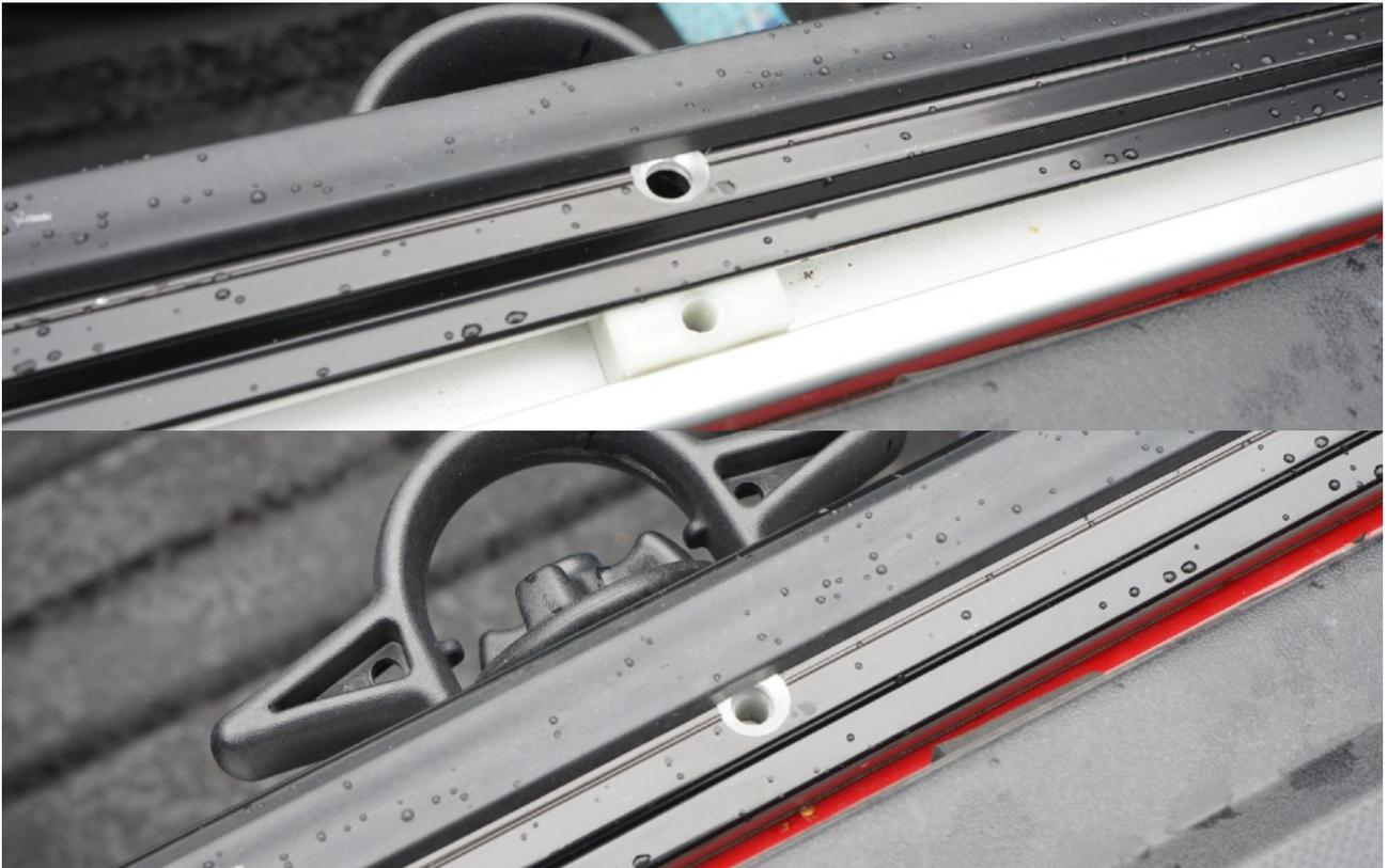
Using Philips size 1 screwdriver introduce all bolts. Keep them loose at first, once you have all bolts introduced, make sure the rail is all the way in and level then tighten evenly.
