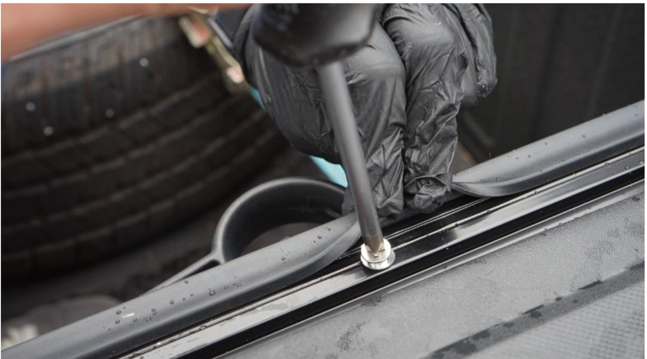
Clean and degrease the front of the bed edge. Place the long rubber seal in place. Cut to length if necessary.
