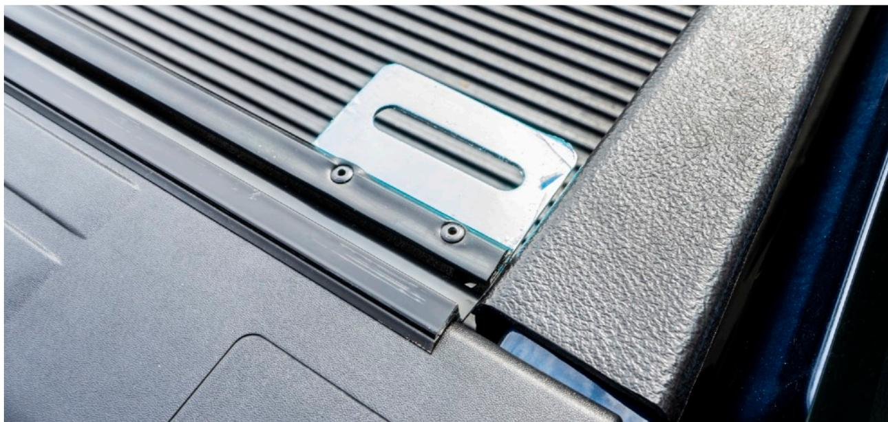
Install side rails to the bed edges using three clamps on each side as shown in the picture. Make sure the edges of the inner clamps are well covered by provided foam stickers.
