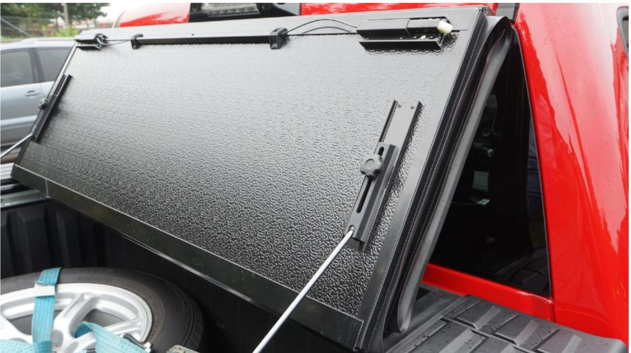
Inspect the seals around the bed cover. Adjust if necessary. New seals might require some time to be fully seated.
