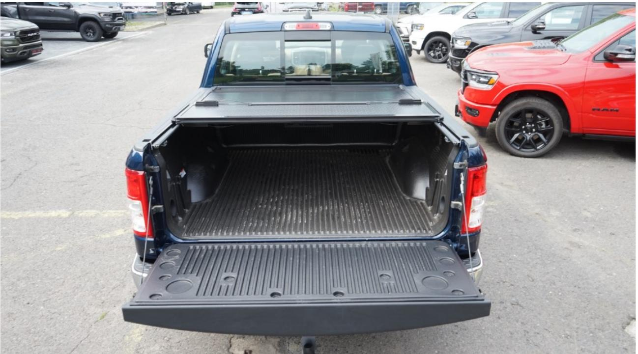
Locate the part of the cover that will be touching the back of the cab once folded. Clean and degrease. Install provided foam bump stop. Depending on your vehicle you can cut two parts to have the cover well supported and your vehicle protected.
