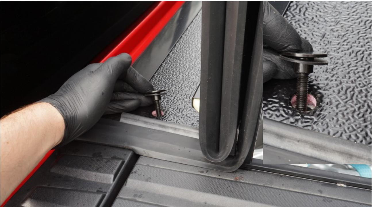
From underneath install large washers and nut as shown in the picture. Introduce a few rounds of threads. Do not tighten fully just yet.
