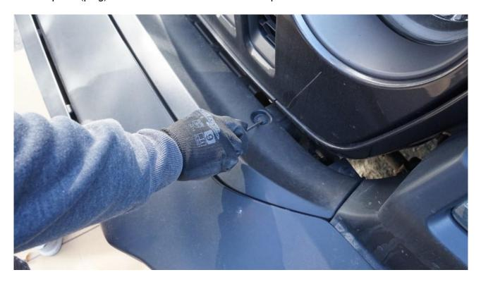
The same trim piece is also held by white clips from inside the bumper. Release them by pinching them and pushing up. Use long needle nose pliers for best access. Gently pulling the masking bar upwards also helps in this task.
