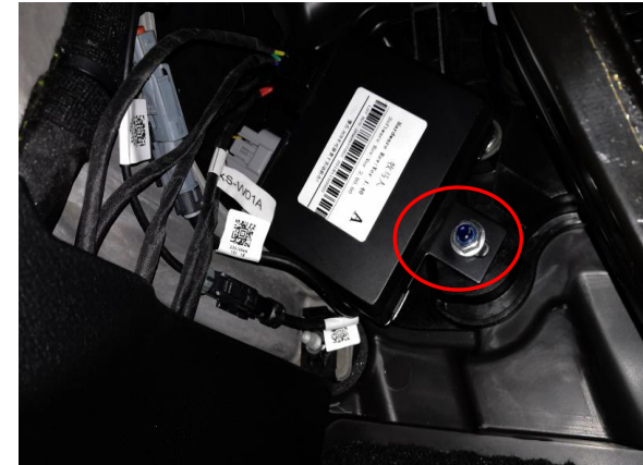
9) Fix the ECU with M8 Screw
