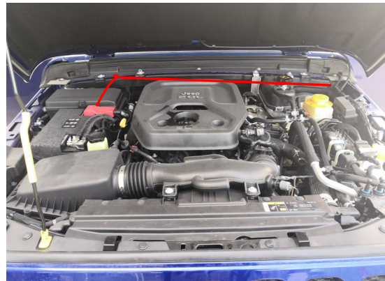
5) Connect the positive pole to the battery
