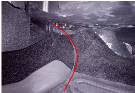
11) Link Another motor line to co-drive side
