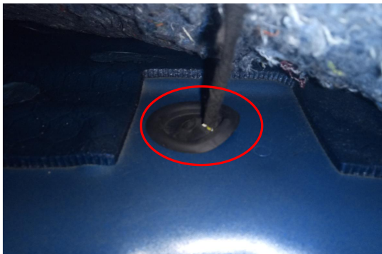
10) Link one motor line from the carpet to the chassis
