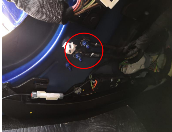
7) Connect negative pole to this place
